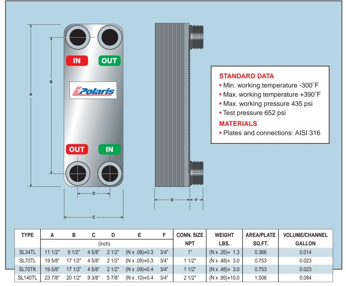
(N = number of plates) (Solder connection available.) Higher working temperatures/pressures available.
